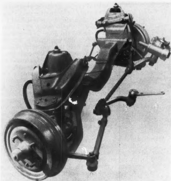
The detachable front suspension unit.
